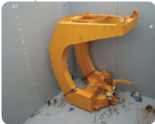
The stacker-reclaimer C-Frame in the Corella Arrow and lashing underway in South Korea.
