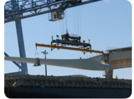
A quay crane at Fraser Surrey Docks unloads a wind turbine blade from ocean carrier to barge.
