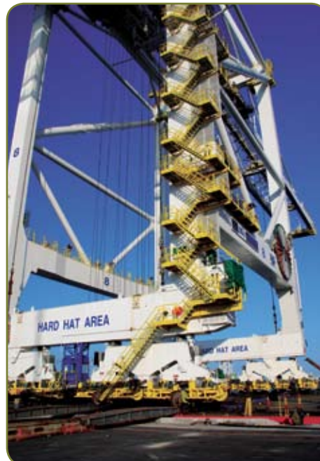
Dual-hoist cranes can hoist two 40-foot containers or four 20-foot containers at the same time. Photo Credit: Jeff Edgar
